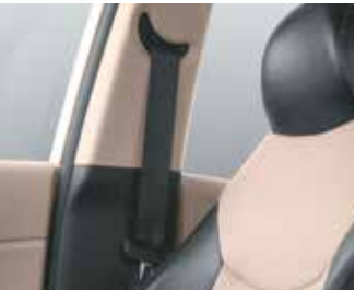
Front Seatbelt Pretensioners with load limiters
